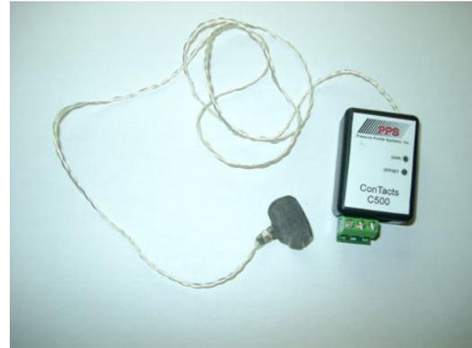
Figure 5: Capacitance sensor with conditioning unit.
